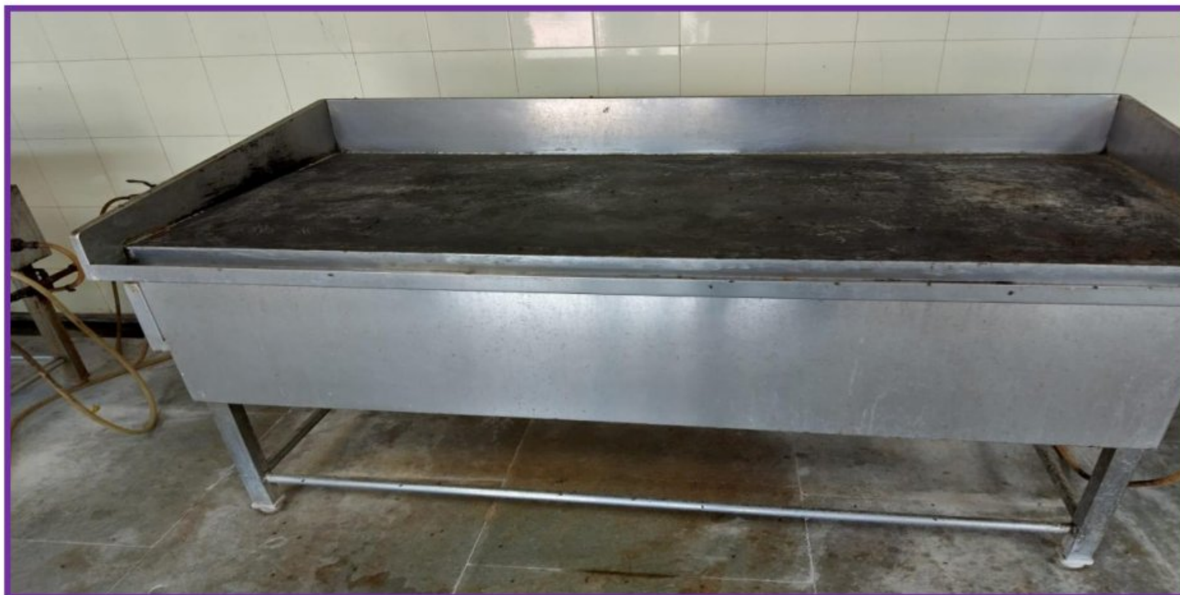
Dosa Maker connected to Biogas plant
